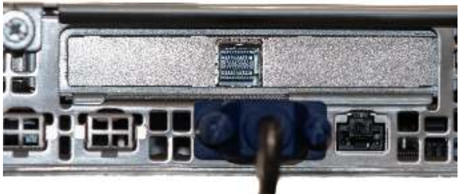
Figure 1-6 SAS tape-out adapter
